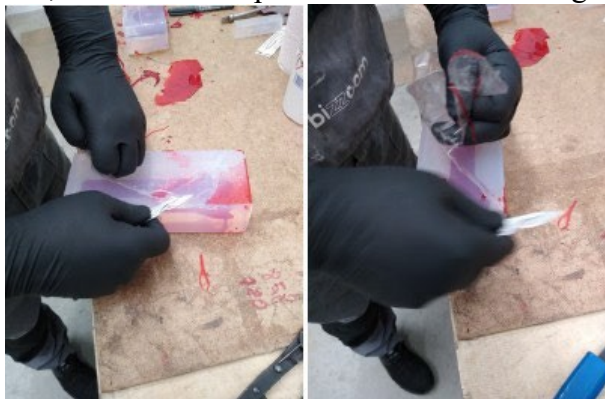
Fig. 3.25 Removing the adhesive tape
