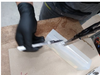
Fig. 3.20 Removing the R1 physical model from the mold
