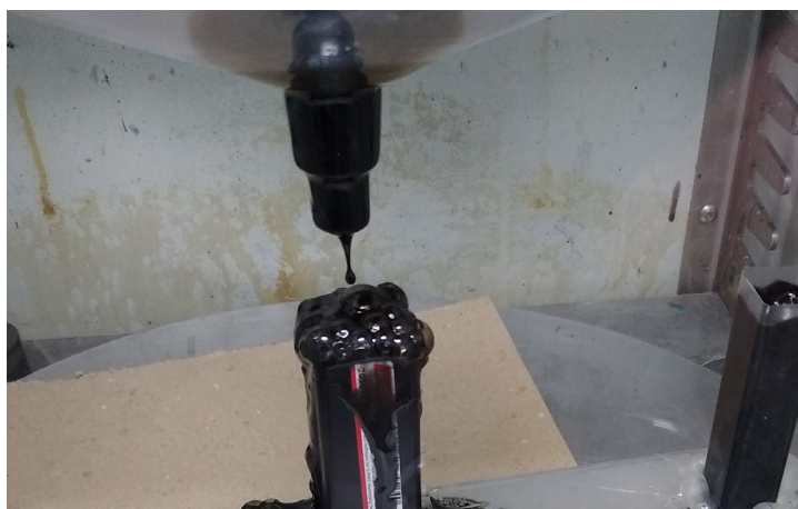
Fig.3. 36 Vacuum degassing of the R1 mold
