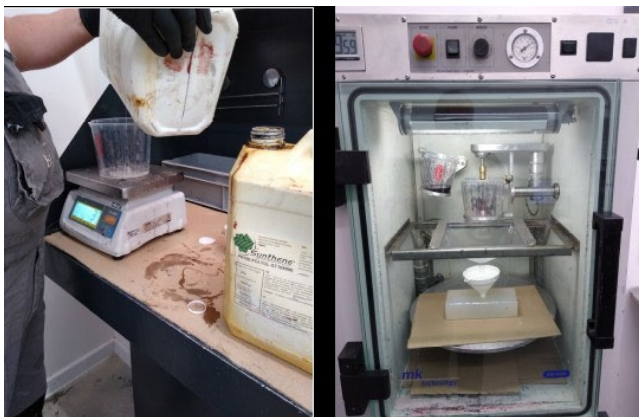
Fig. 3.34 Weighing the individual components of the mixture and their insertion in the vacuum chamber
