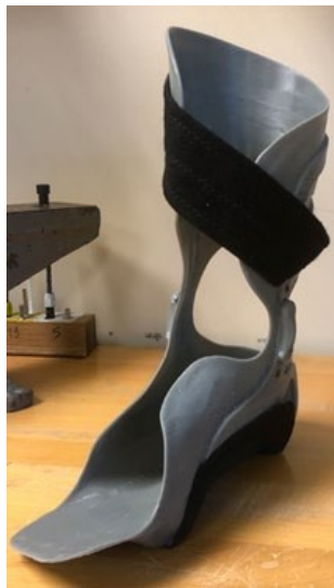
Fig 2.3. Individualized orthosis printed with FDM technology [www 07].
