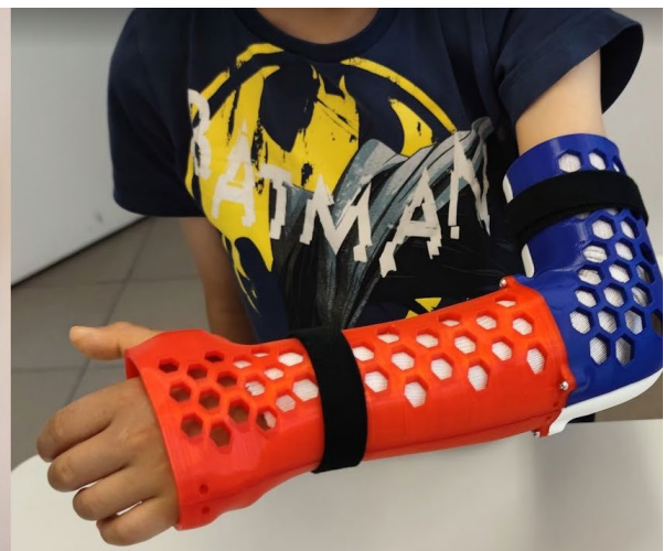
Fig 3.23. Manufactured orthosis (PLA) during use.
