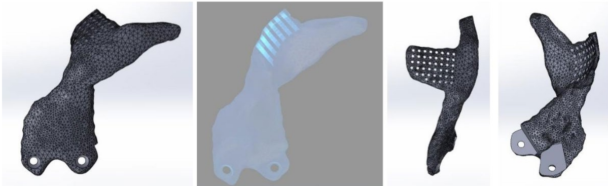
Fig. 3.6. Creating 2 fixing holes with 2.6 mm diameter and perforate the orbital surface of zygomatic bone with 32 holes with 1.1 mm diameter
