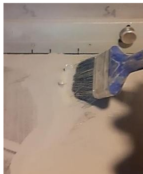
Fig. 3.23. Cleaning the implant of powder
