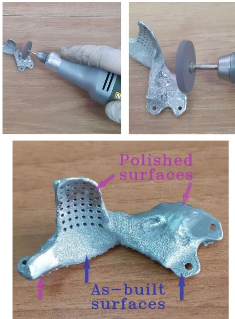
Fig. 3.24. Biax micro-motor used to polish the implant
