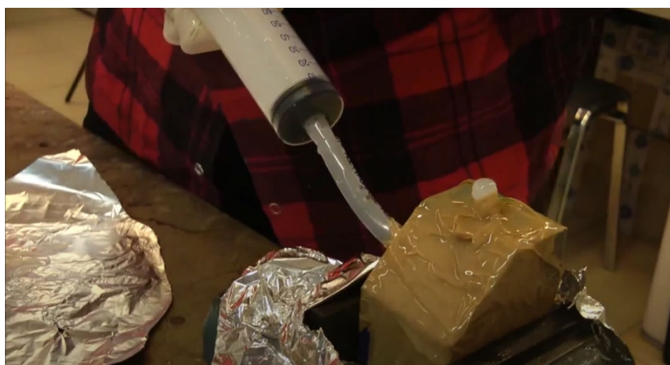
Figure 23. The resin casting process
