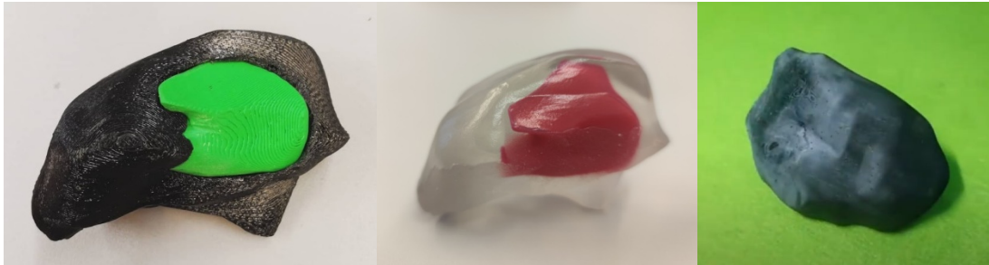
Figure 21. Hard 3D printed models of tongue with cancer – FDM, PolyJet and SLA technology
