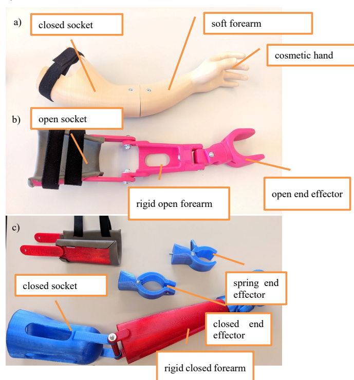
Figure 17. Modular construction of the prosthesis
