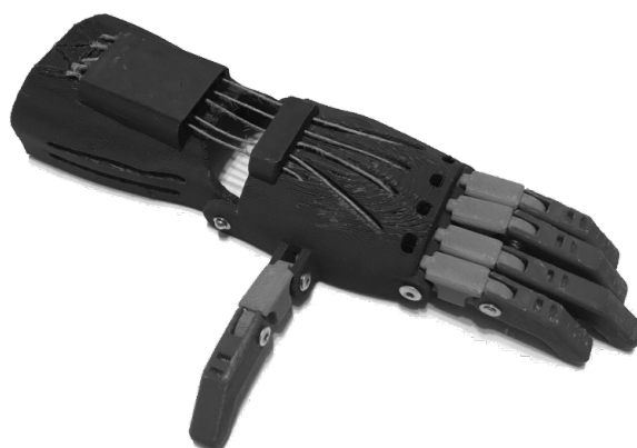
Figure 14. RoboHand prosthesis made of ABS material
