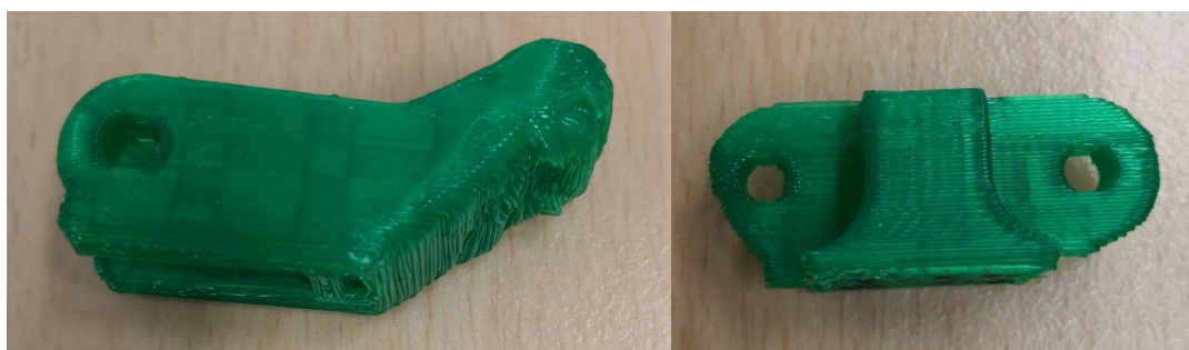
Figure 15. Examples of error in the manufacturing process
