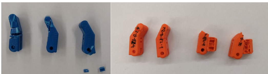
Figure 21. Result of strength test - fingers
