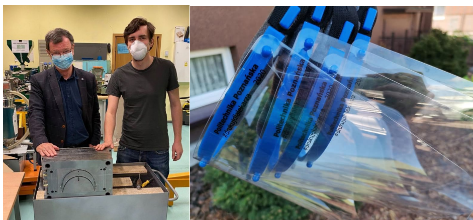
Figure 21. Professors of PUT with injection mold for the face shield and examples of face shields manufactured with this technology
