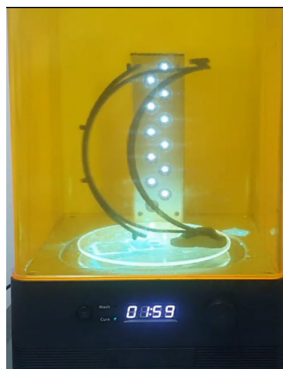
Figure 16. Anycubic SLA post-curing machine – post-curing of the shield base
