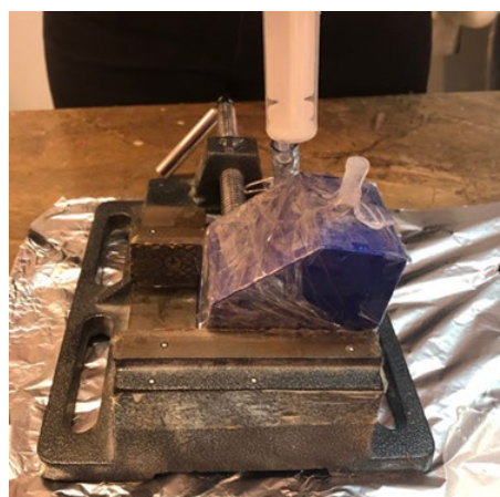
Figure 28. A mold prepared for the casting process
