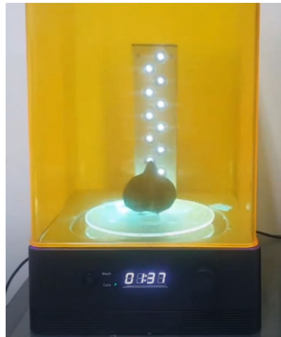
Figure 23. Anycubic SLA post-curing of the tongue model
