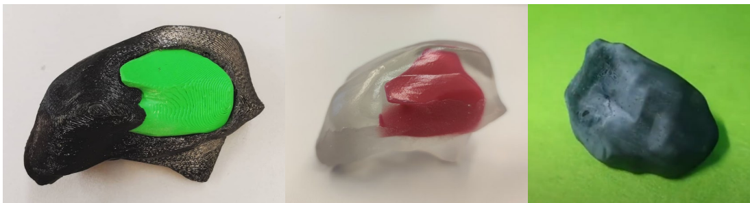
Figure 26. Hard 3D printed models of tongue with cancer – FDM, PolyJet and SLA technology
