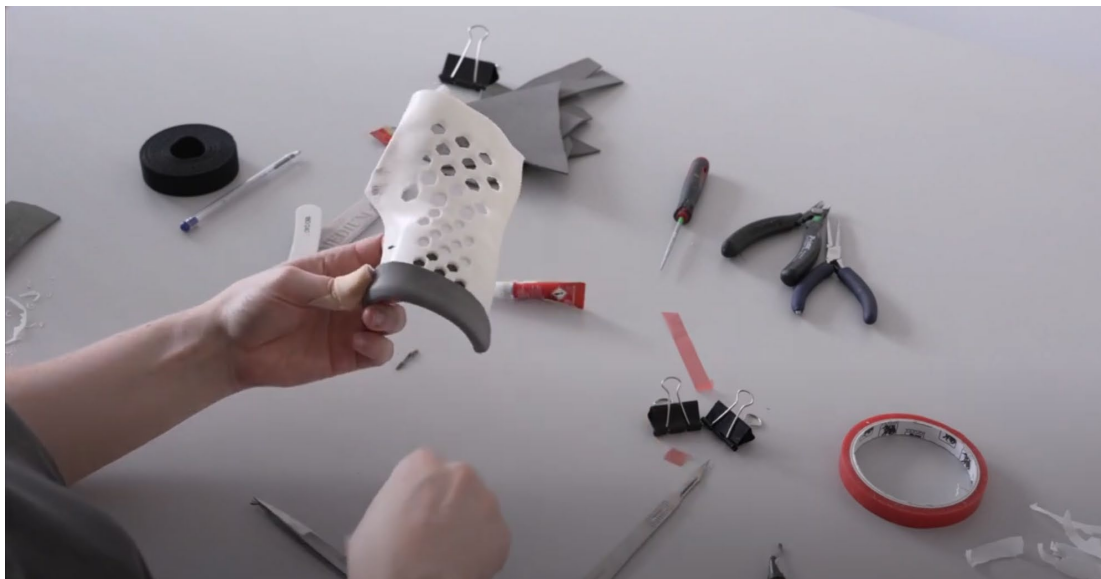
Figure 19. Post processing of the orthosis (support removal, lining with foam etc.)
