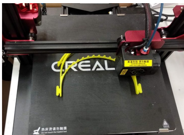
Figure 7. 3D Printing of face shields using generic FDM printer
