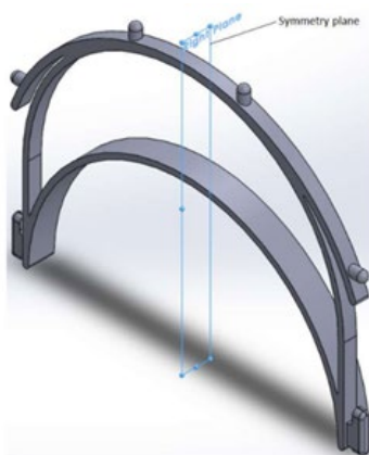
Fig. 15. Three-dimensional model of the face shield base (frame extracted from the recording of the CAE webinar)
