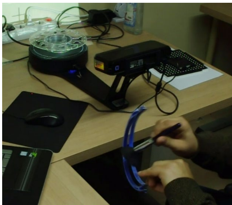
Figure 12- Pre-processing the face shield for 3D scanning
