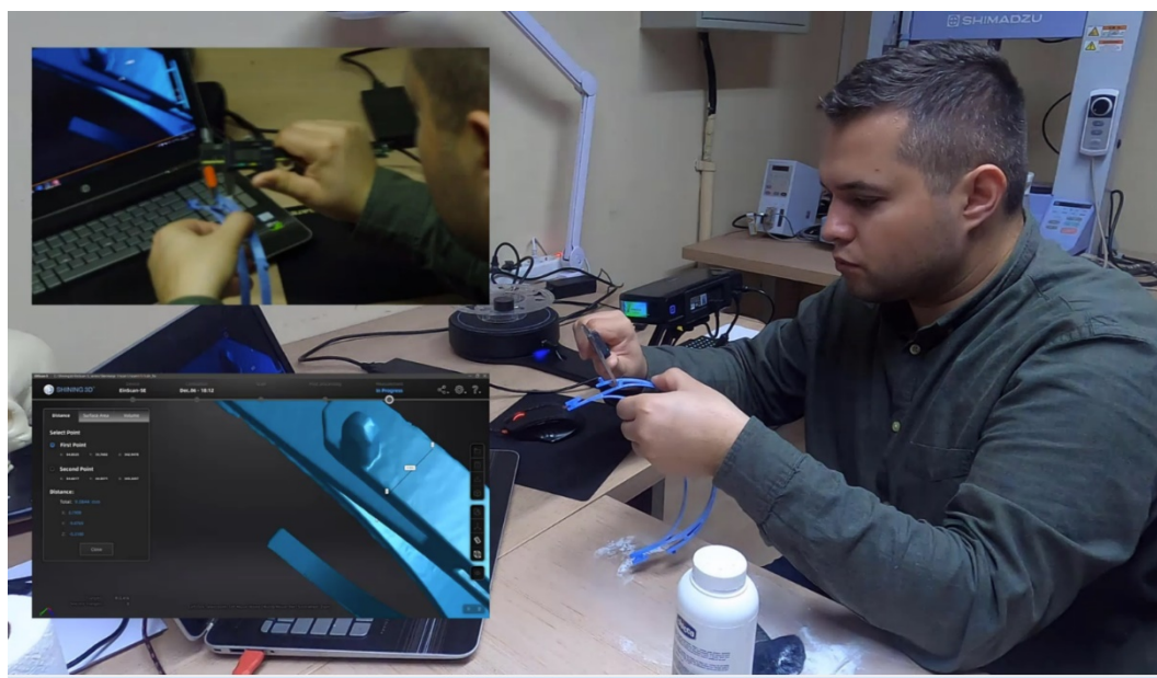
Figure 14- Comparing the scan model dimensions to those of CAD model
