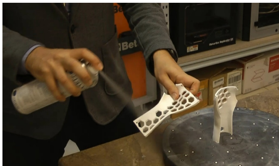
Figure 5- Pre-processing the orthosis for 3D scanning
