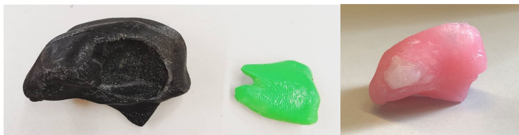
Figure 6. Model of a tongue with cancer – hard 3D print (left) and soft casting in a 3D printed mold (right)
