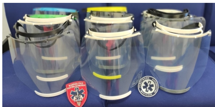
Figure 8. 3D Printed assembled face shields for a hospital
