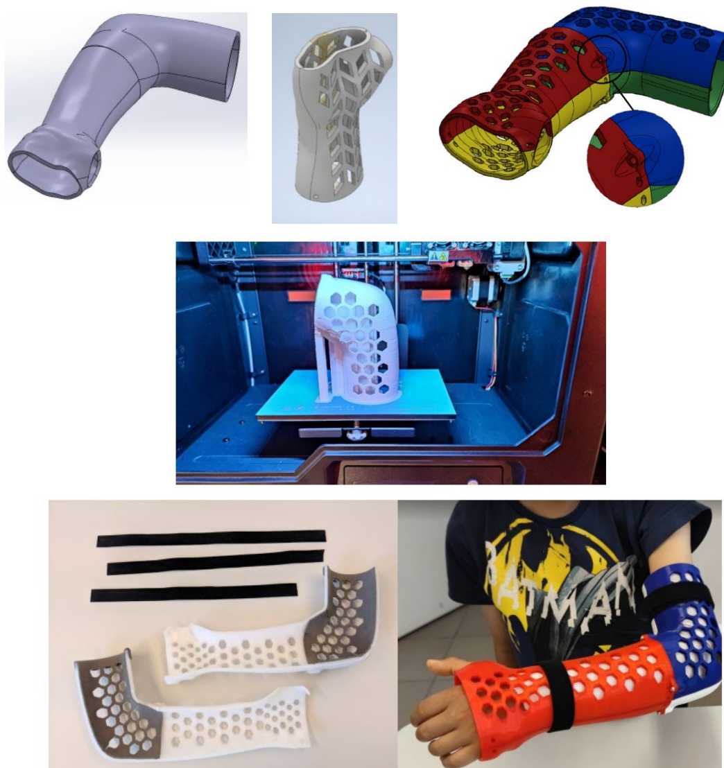
Figure 11. Designing and 3D printing process of orthosis made by FDM and Reprap 3D printing technologies from Nylon and ABS material
