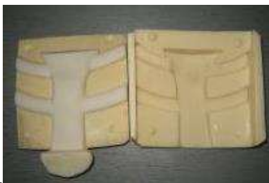
Figure 8.12 Implant cast in a mould before finishing
