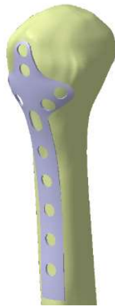
Figure 9.6 Assembly of the plate solid model and surface model of the test humerus bone
