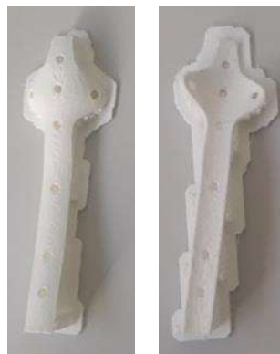
Figure 9.7 Creation of personalized 3D cloverleaf plate
