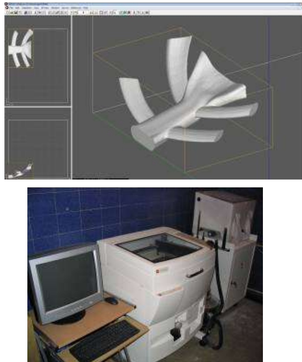
Figure 8.7 Model in ZPrint software (left) and 3D printer (right)
