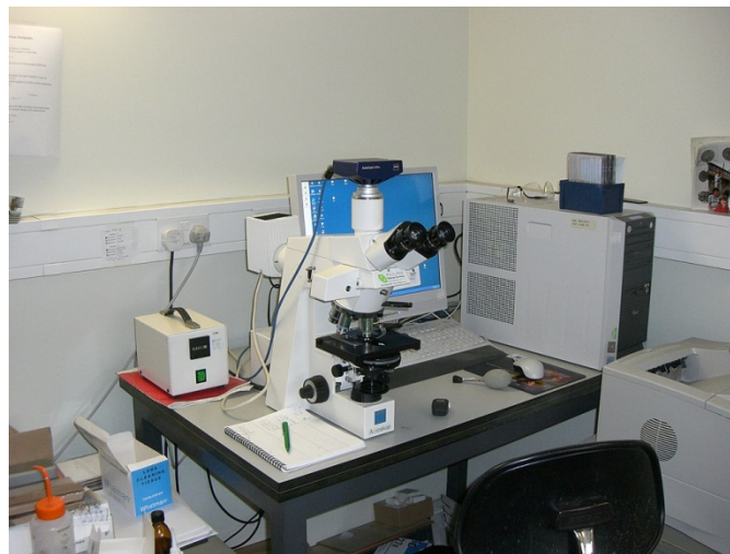
Figure 5.9. A modern optical microscope with a mercury bulb for fluorescence microscopy. The microscope has a digital camera which is connected to a computer [109].
