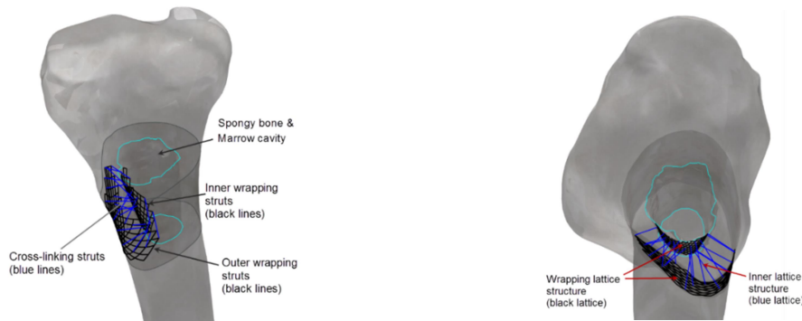
Fig. 3.19. Design concept of ASLS (Anatomically Shaped Lattice Scaffold) [STO13]
