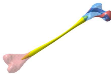
Fig. 4.10. Zones created inside the solid model of the femur, which are later used in meshing process (approach 2). Zones are created to approximately represent the segments of different trabecular bone density. The zone representing cortical bone is omitted for clarity [KOR10]
