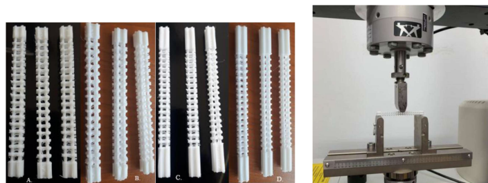
Fig. 3.7. Printed samples made by FDM: A-circular porous structure for flexural tests, B-circular porous structure for tensile tests, C-circular porous structure for flexural tests, and D-square porous structure for tensile test
