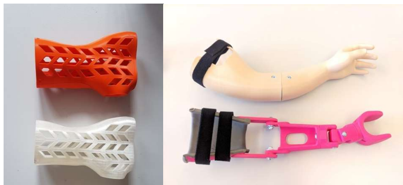
Figure 3.45 Examples of orthopaedic supplies made by 3D printing on the basis of 3D scanning [37]
