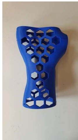
Figure 3.64 3D printed orthosis example
