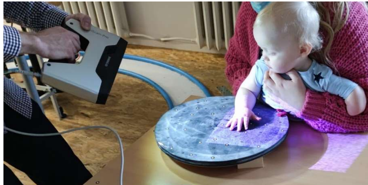
Figure 3.46 Manual 3D scanning of patient limb (EinScan Pro)
