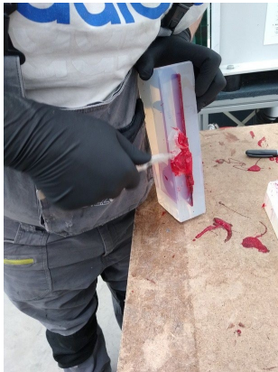
Fig. 3.27 Removing the R1 casting from the mold
