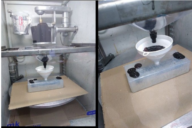
Fig. 3.35 Preparing the mixture and pouring it into the mold placed in a vacuum chamber
