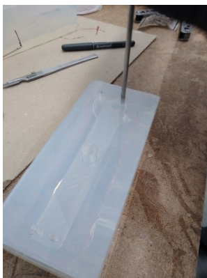
Fig. 3.22 Creation of five vent holes in the mold
