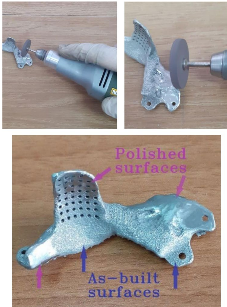
Fig. 3.24. Biax micro-motor used to polish the implant
