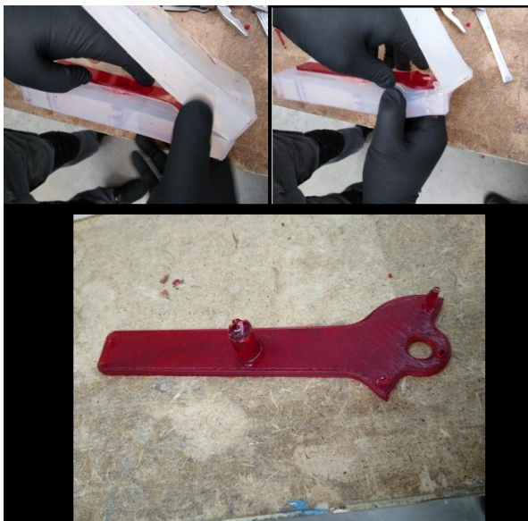
Fig. 3.30 Removing the R2 casting from the mold
