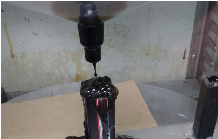
Fig.3. 36 Vacuum degassing of the R1 mold
