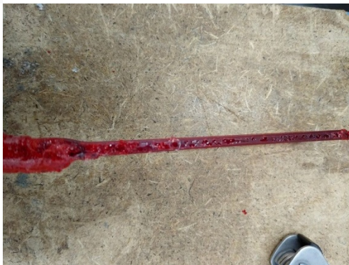
Fig. 3.29 Unexpected bubbles in the casting R1
