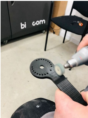
Fig. 3.39 Grinding of castings after removing the inlet and vent
