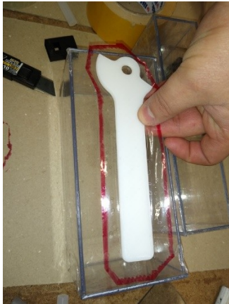
Fig. 3.15 Duct tape used for materializing the separation surface on the R2 model
