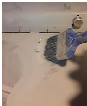
Fig. 3.23. Cleaning the implant of powder
