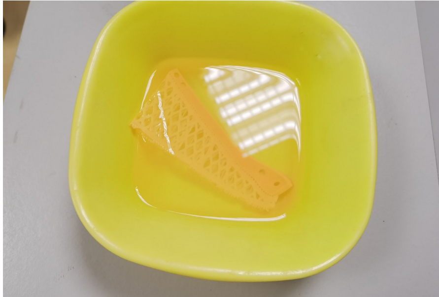
Figure 5.52. Washing of part in isopropyl alcohol
