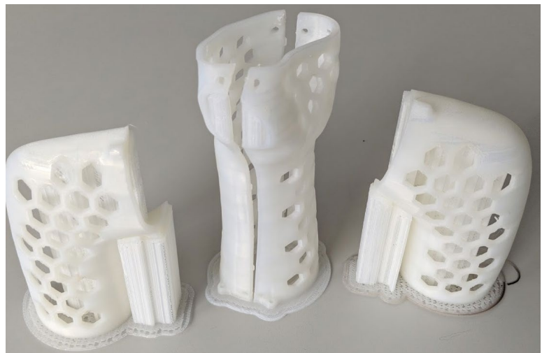
Fig 3.21. Manufactured orthosis parts – nylon
