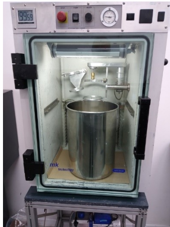
Fig. 3.17 Removing air bubbles and other gaseous impurities from the mixture of silicone and hardening agent in a vacuum chamber
