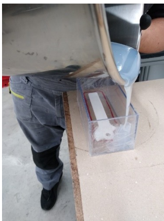
Fig. 3.18 Pouring the silicone mixture into the case
