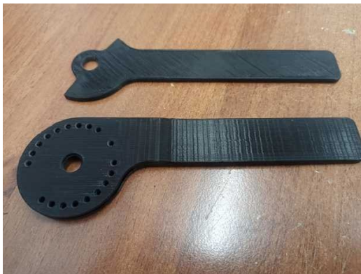
Fig.3.40 A set of black R1 and R2 parts after cleaning the castings, without noticeable defects
