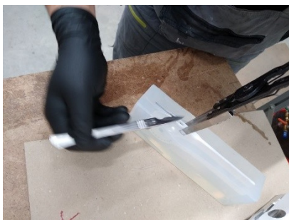
Fig. 3.20 Removing the R1 physical model from the mold
