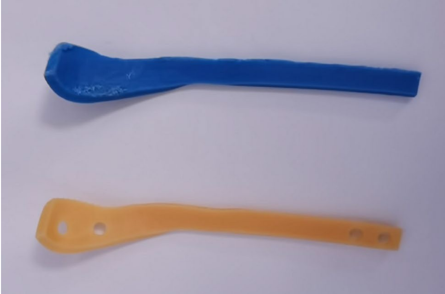
Figure 6.56. Printed part by FDM (up) and Stereolithography (down)
