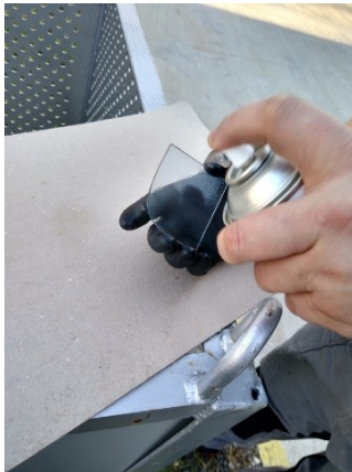
Fig. 3.23 Application of separator on the plexiglass
