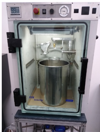
Fig. 17 Removing air bubbles and other gaseous impurities from the mixture of silicone and hardening agent in a vacuum chamber
