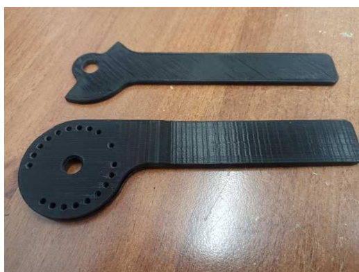
Fig. 40 A set of black R1 and R2 parts after cleaning the castings, without noticeable defects
