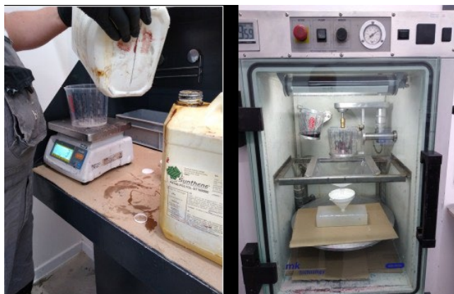
Fig. 34 Weighing the individual components of the mixture and their insertion in the vacuum chamber
