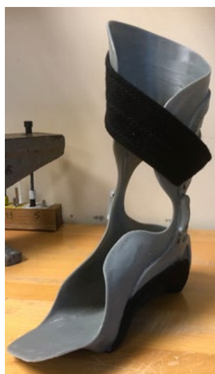
Fig 3. Individualized orthosis printed with FDM technology [www 07].
