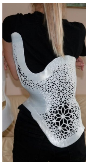
Fig 4. Individualized back brace printed with FDM technology [www 08].
