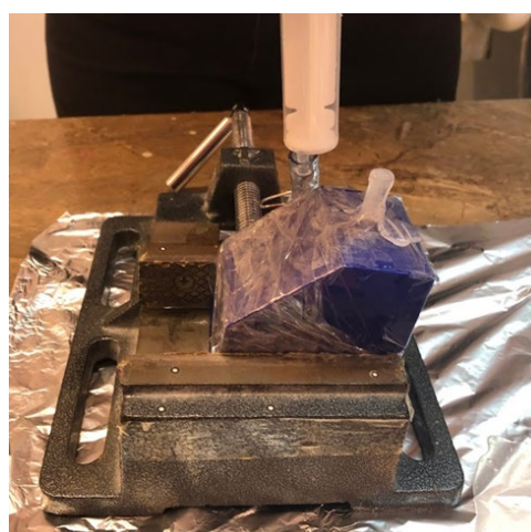
Fig. 3.22 A mold prepared for the casting process
