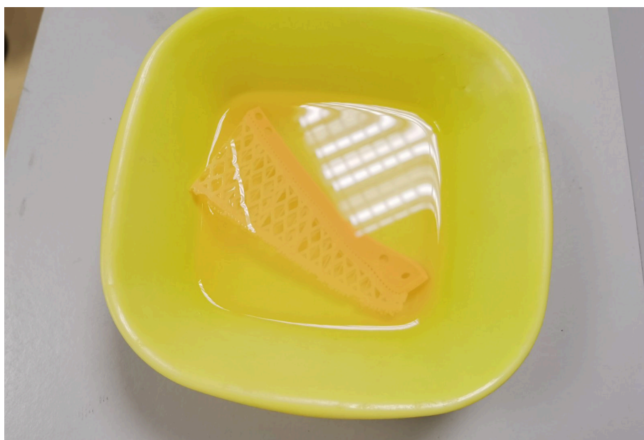
Figure 52. Washing of part in isopropyl alcohol
