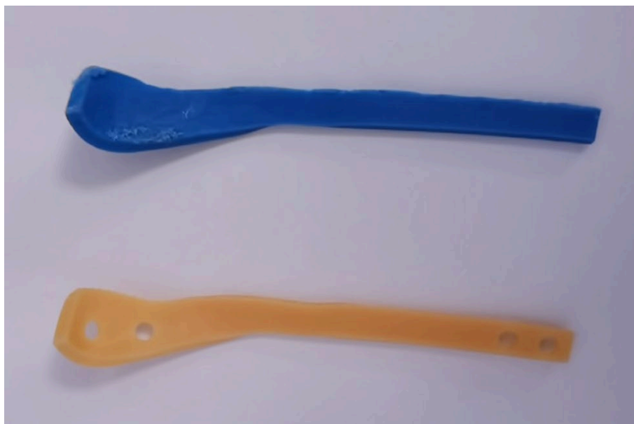
Figure 56. Printed part by FDM (up) and Stereolithography (down)
