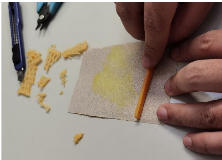
Figure 54. Postprocessing of 3D printed part
