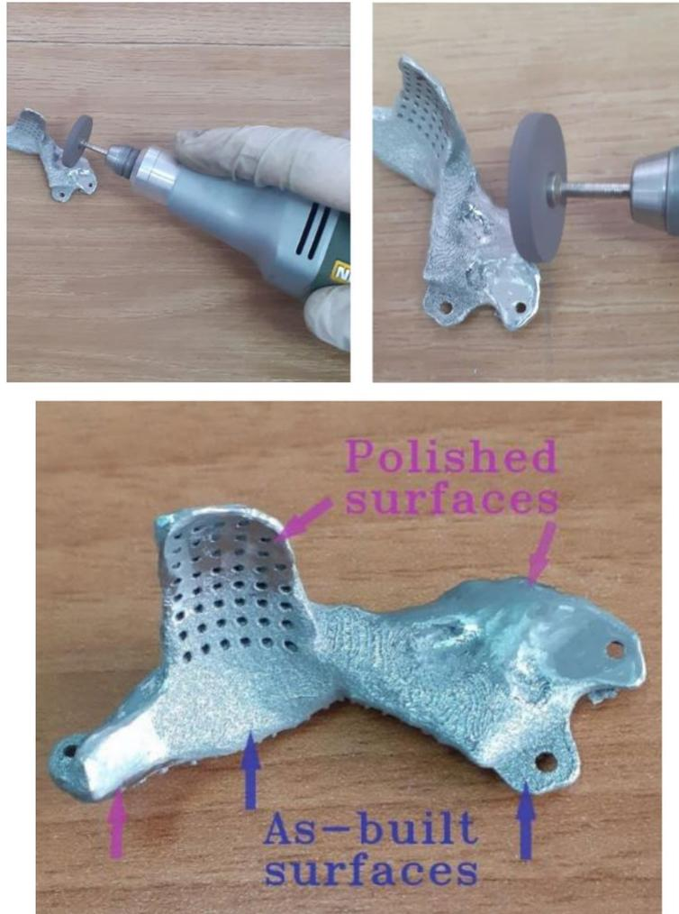
Fig. 3.24. Biax micro-motor used to polish the implant
