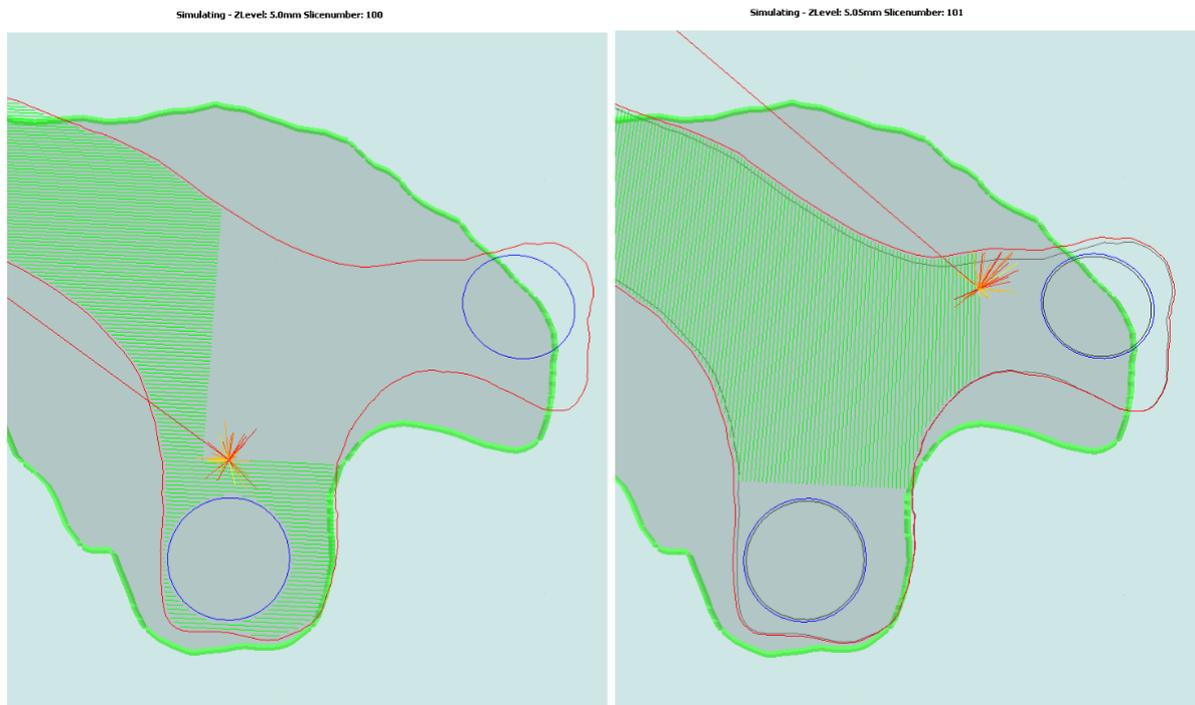
Fig. 3.15. SLM simulations at 100 and 101 slices
