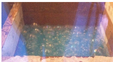
Figure 5.6. Removing the air bubbles from the mould
