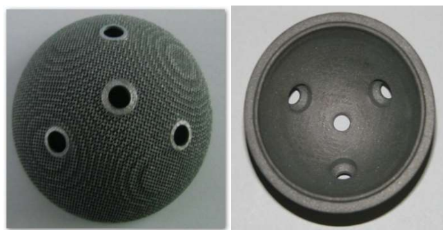
Fig. 4.23. Customized implant produced from Ti6Al4V powder on the SLM 250 HL machine
