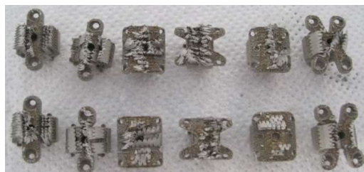
Fig. 3.70. Cervical disc implants manufactured by SLM (before the supports were removed)
