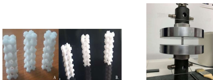
Fig. 3.6. Printed samples made by FDM for compressive tests: A-circular porous structure, B-square porous structure
