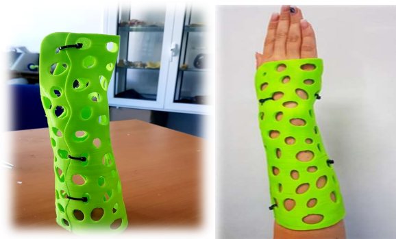
Fig. 2.9. Customized arm orthosis produced by FDM
