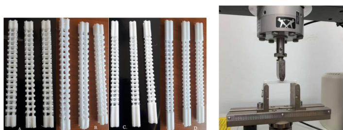
Fig. 3.7. Printed samples made by FDM: A-circular porous structure for flexural tests, B-square porous structure for flexural tests, C-circular porous structure for tensile tests, and D-square porous structure for tensile test
