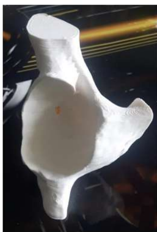
Fig. 3.18. 3D printed model of the pelvic bone
