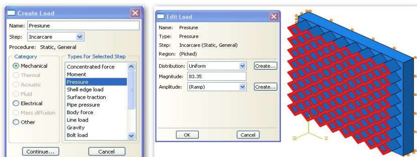
Fig. 4.20. Pressure load applied in the analysis
